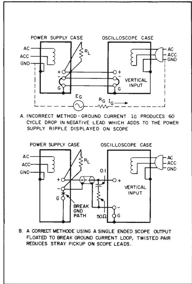
Figure 5-3. Ripple and Noise, Test Setup
