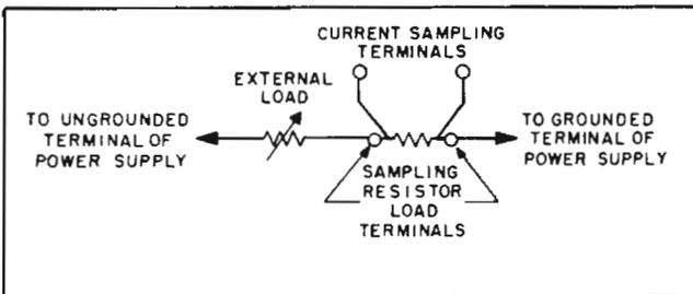
Figure 5-1. Current Sampling Resistor Connections
