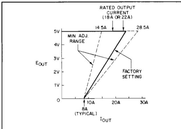
Figure 3-6. 5V Output, Current Limit Characteristics
