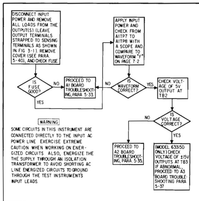
Figure 5-6. Circuit Board Isolation Procedure
