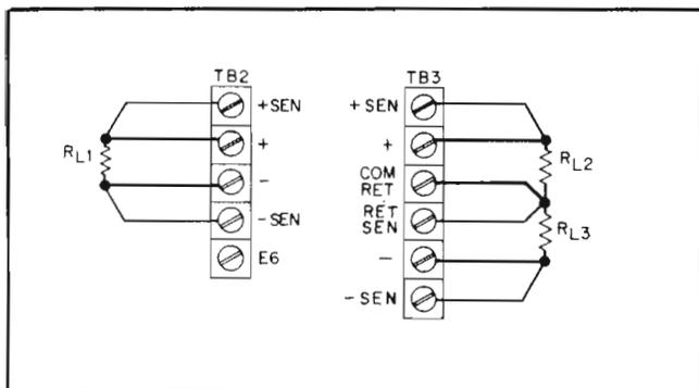
Figure 3-3. Load Connections, Remote Sensing
