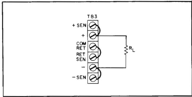
Figure 3-2. Single Load, Local Sensing
