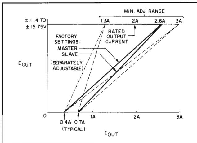
Figure 3-7. Model 63315D, Dual Output, Current Limit Characteristics
