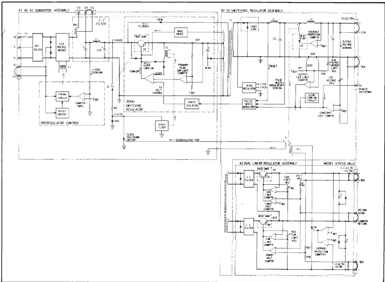
Figure 4-1. Models 63005C and 63315D Simplified Schematic Diagram
