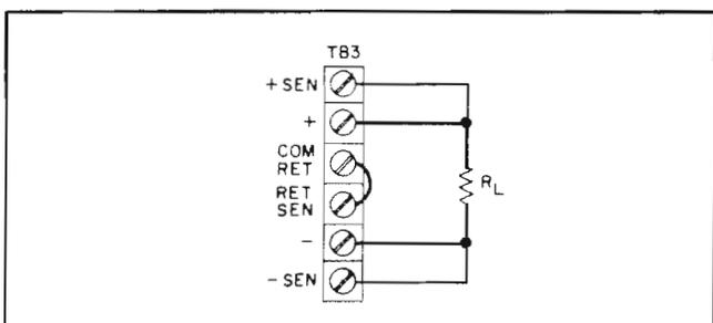
Figure 3-4. Single Load, Remote Sensing
