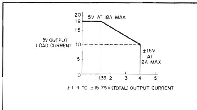
Figure 3-5. Load Sharing Tradeoff, Model 63315D
